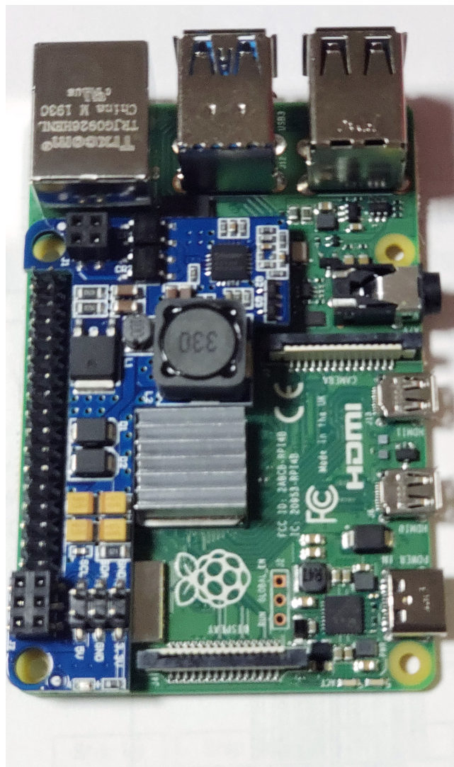
3. Peel off the backing and install heat sink on RPi
